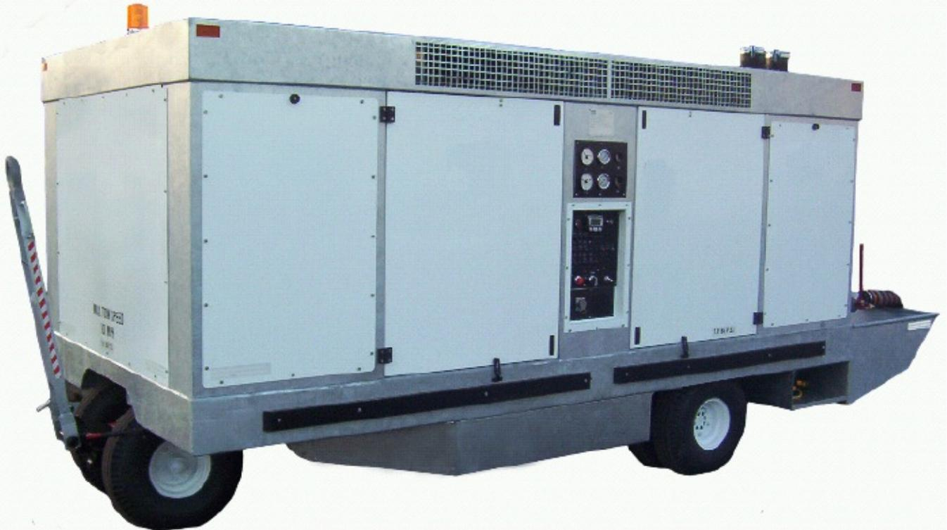
**The ASU-600 Series** is a line of truck or trailer mounted continuous flow jet engine starting units, producing 180-300 ppm of airflow at up to 40 psig pressure.
